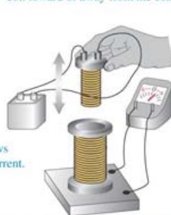
(c) Moving a second, current-carrying coil toward or away from the coil
