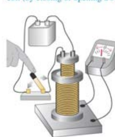
(d) Varying the current in the second coil (by closing or opening a switch)
